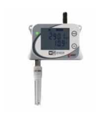
Sensors with WiFi interface are designed to measure the temperature, relative humidity, CO2 and atmosperic pressure with a connected probe (included in delivery).
