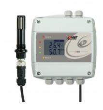
Compressed-air ambient humidity, temperature Ethernet sensor with two relay outputs. T+RH probe from hard anodized duralumin for compressed air up to 25 bars with cable.
