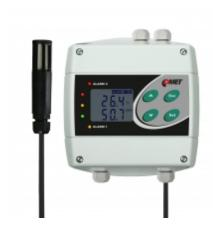
Humidistat, thermostat with two relay outputs. Outdoor, indoor use. Relative humidity, temperature probe on a cable. Measured values are also converted to other humidity interpretation: dew point temperature, absolute humidity, specific humidity, mixing ratio, specific enthalpy.
